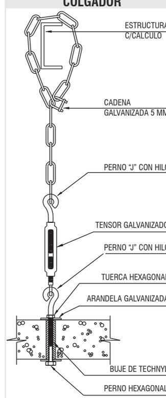
Labels: ESTRUCTURA C/CALCULO, CADENA GALVANIZADA 5 MM, PERNO "J" CON HILO, TENSOR GALVANIZADO, PERNO "J" CON HILO, TUERCA HEXAGONAL, ARANDELA GALVANIZADA, BUJE DE TECHNYL, PERNO HEXAGONAL.
