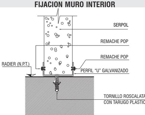
Labels: SERPOL, REMACHE POP, REMACHE POP, PERFIL "U" GALVANIZADO, TORNILLO ROSCALATA CON TARUGO PLASTICO, RADIER (N.P.T.).
