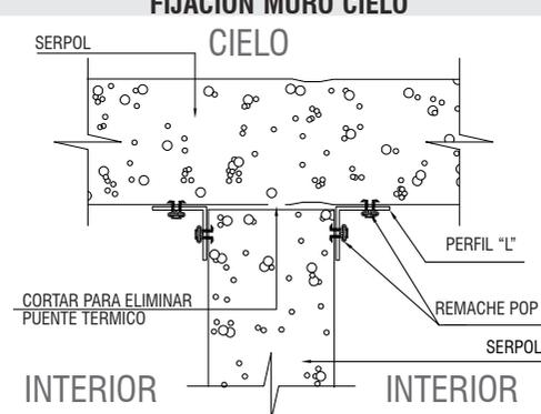
Labels: SERPOL, CIELO, PERFIL "L", REMACHE POP, SERPOL, INTERIOR, INTERIOR, CORTAR PARA ELIMINAR PUENTE TÉRMICO.
